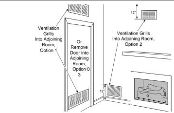
Figure 2 - Ventilation Air from Inside Building
